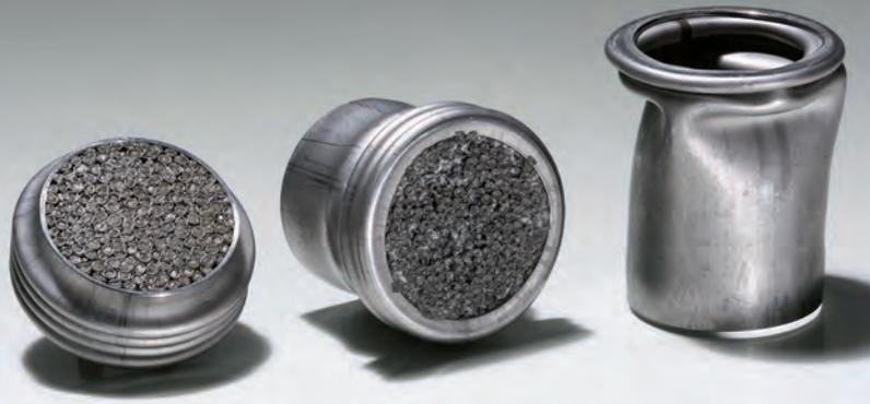
By adjusting the density and the basic material of the hollow sphere structure the needed mechanical, thermal and corrosive properties are tailored. Furthermore, by adjusting the kinetic energy absorption of the hollow sphere structure the required volume of the crash absorbers may be determined. The required volume of such parts may be lowered considerably in comparison to an unfilled absorber.
