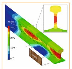
Fig. 1 Temperature distribution on a railway track with lateral heater
