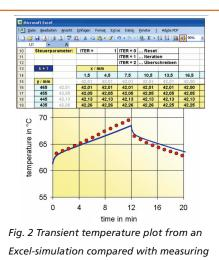
– by means of an air flow. Based on the measurement of heat generation rates in a single cell depending on the charging electric current a qualified flow and heat transfer model was created and used to simulate various operating conditions.
