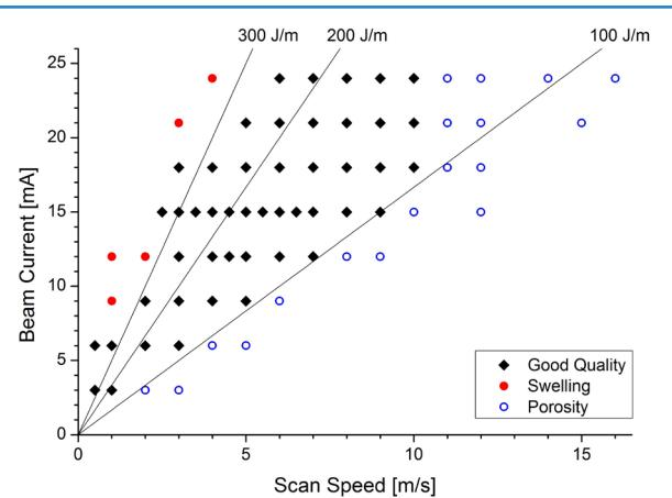
Fig. 2 Process window for SEBM of Ti-6Al-4V. Blue circles mark samples with more than 1% porosity, red circles mark considerable swelling at the surface.
