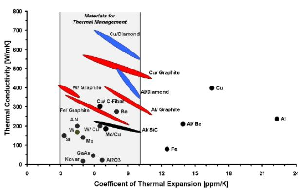
*Fig. 1 Property profile of different composites for passive heat sinks.*
