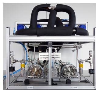
Fig. 3 Two-stage metal hydride compressor testing unit (max. 200 bar, 400 °C).
