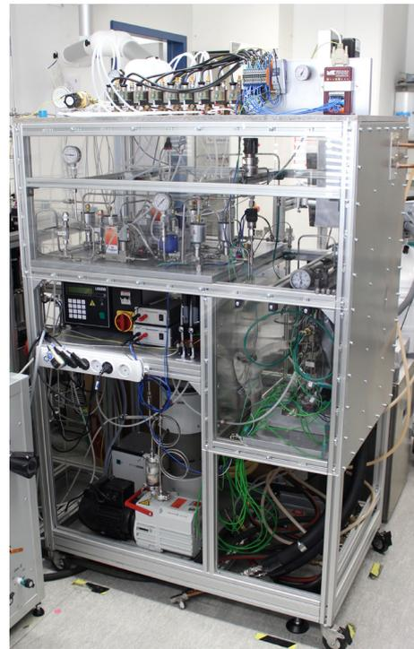
Fig. 5 Test rig for metal hydride tank evaluation.
