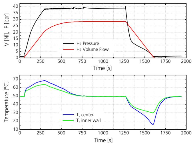
Fig. 6 Fast loading and unloading characteristics of metal hydride composite materials (cf. Fig. 4). Hydrogen is absorbed and desorbed in a few minutes.
