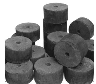
Fig. 4 Metal hydride composites for dynamic sorption processes.
