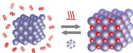
Fig. 1 Metal hydride formation (schematics)
