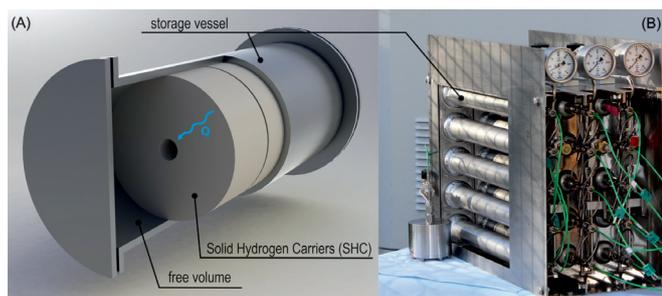
Fig. 2 A: Schematic drawing of a SHC storage module.
