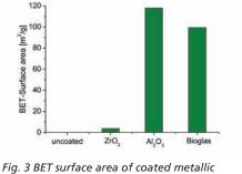
hollow spheres after pyrolysis at 800 °C
