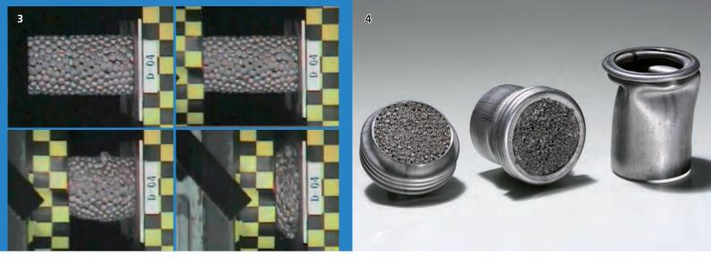
By adjusting the density and the basic material of the hollow sphere structure the needed mechanical, thermal and corrosive properties are tailored. Furthermore, by adjusting the kinetic energy absorption of the hollow sphere structure the required volume of the crash absorbers may be determined. The required volume of such parts may be lowered considerably in comparison to an unfilled absorber.
