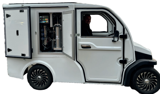
Light electric vehicle using POWERPASTE
