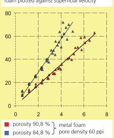
Pressure losses are measured by means of pressure transducers available for gases and liquids with different measuring ranges. To evaluate and process the results, various options are possible:
