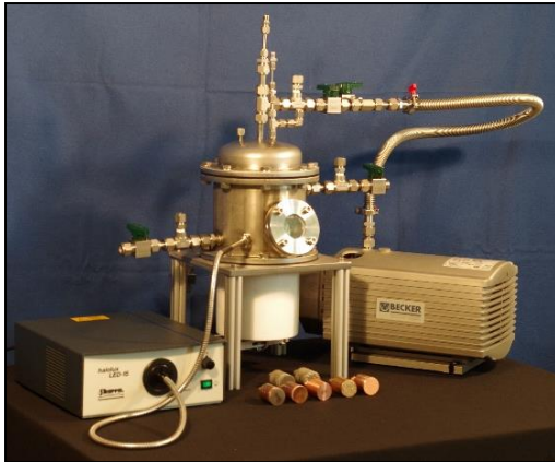
Test rig for metrological characterization of evaporator surfaces
