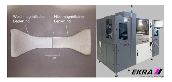
Test structure of a hybrid material produced by screen printing, consisting of a soft magnetic alloy and a non-magnetic alloy (left). Screen printing facility of EKRA Automatisierungstechnik GmbH at Fraunhofer IFAM Dresden, which was used to produce the hybrid structures (right).
